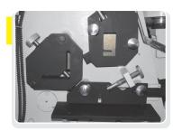
Angle, channel & Flat stations are equipped with tools. Angle station doesn't require any blade change for any size of angles. Flat station can be used for shearing flats as well angle 45° cuts. Channel station can cut different sizes of Channel, Round bar, square bar, I- section & T-section by changing the dies. The die change is quick & easy.
