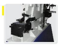
The notching station is used for notching of plate, Flats, Angles and Channels. Different types of Notching operations can be done to suit various structural joints.
