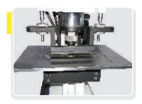
The punching station is suitable for punching on plates, Flats, Angle and channels. It is equipped with quick release type Punch & self aligned dies for various punching shapes like round, square, capsule or oval shapes. The die change is quick & easy. Optional press brake tool & "V" die can be used for flats & bus bar bending.
